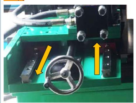
1. In the front and rear direction, the large load-bearing slide rail + screw rod, and the worktable can move back and forth to facilitate the corner cutting of mesh with different widths.
