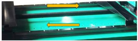
2. Left and right direction, large load-bearing slide rail + screw rod, the worktable can be moved left and right, which is convenient for mesh corner cutting of different lengths
